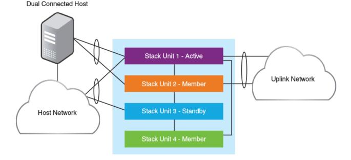
In the figure, redundant links are going to both the uplink network and the downlink network from different units of the stack. At any point during the upgrade, the uplink and downlink connectivity is maintained. The following software features are used to provide link redundancy:
